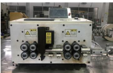
Automatic Cable Cutting & Stripping Machine
