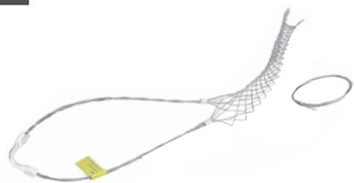
Support Grips distribute the weight of vertical drops and sloping runs over the length of the grip to protect the cable from damage.
